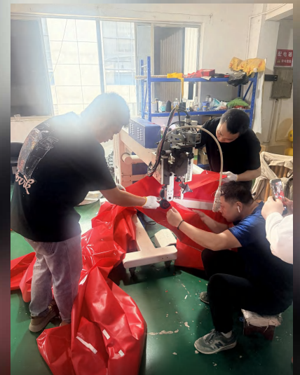
Seam welding at our factory
